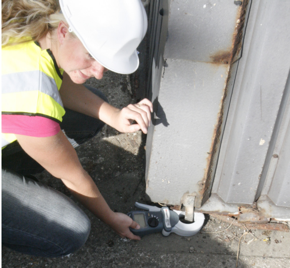
An example of Clamp-On testing using the DET14C and DET24C
