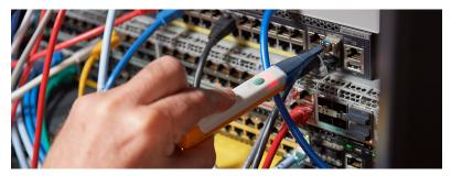
Determine if a transceiver is operational. FiberLert can detect fiber signals without making contact.
